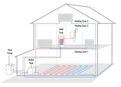
The WPM2004 Plus Heat Pump Manager allows Dimplex LA MS air source heat pumps to provide full control over 3 separate heating circuits as well as the preparation of domestic hot water.
